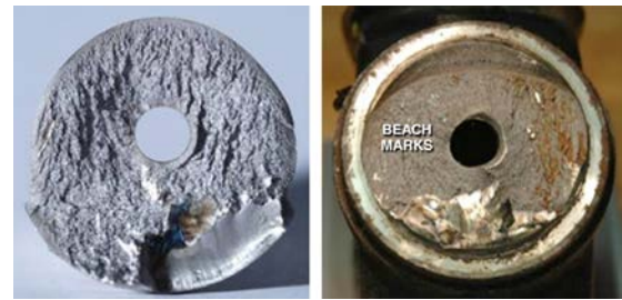
Sudden Overstress Fracture Fatigue Fracture
