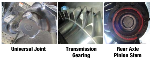
Figure 5 – Fractured Drivetrain Components
